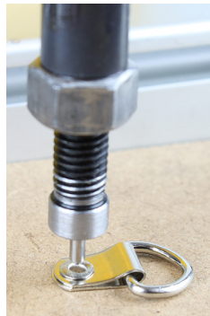
Rivets set flat and smooth both sides
